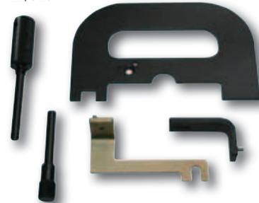
Camshaft sprocket locking device for 16V engines. Essential for removing and installing gear wheels for camshaft.
